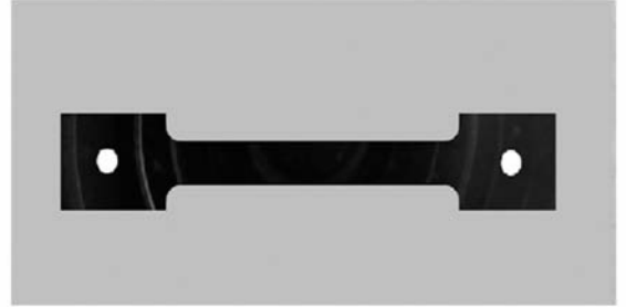
Fig. 2 Specimen with aluminum layer on a PET substrate. The position of circle hole fixes the specimen and the middle of specimen is the observation area.
